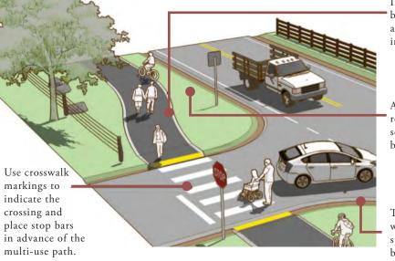
Increasing the separation between the multi-use path and roadway at intersections improves visibility.
